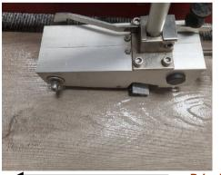
Customer: Dura Composites Test Number: FS10174 Operator: Glenn MacLaughlan Date of Test: January 2023 On Site: Tested at Dura Offices Pendulum Calibration Number: CN642 Pendulum serial number: SK1595 Slider Type :Fours96 Contaminate Description: Water Surface: Dura Deck Inspire - Wren
