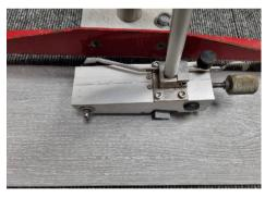
Customer: Dura Composites Test Number: FS10174 Operator: Glenn MacLaughlan Date of Test: January 2023 On Site: Tested at Dura Offices Pendulum Calibration Number: CN642 Pendulum serial number: SK1595 Slider Type :Fours96 Contaminate Description: Water Surface: Dura Deck Inspire - Dove
